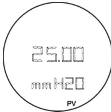
Figure 2.5 – Typical Monitoring Mode Display Showing PV, in this case 25.00 mmH 2 O
