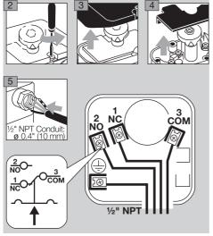
DG..FT, DG..NT: the NO-to-COM connection is interrupted if the pressure drops (contacts 3 and 2 open).
